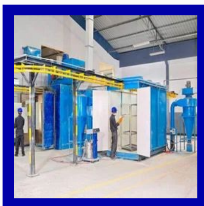
Powder Coating Plant
