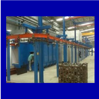
I Beam Conveyor
